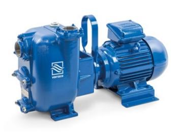
**Product Data** Suction port Threaded - 2" ISO 228 (BSP) Delivery port Threaded - 2" ISO 228 (BSP) Qmax 50 m<sup>3</sup>/h - 833 l/min (220 USgpm) Hmax 52 m (170 ft) Solids handling 15 mm (0.6 ") Motor power 11 kW - 15 HP Motor type **IEC** standard Winding for inverters **Cast iron frame** Motor brand WEG W22 Premium Weight 185 ka
